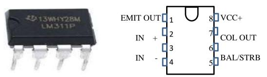
Figure 4 Component of LM311 comparator and pin out diagram
