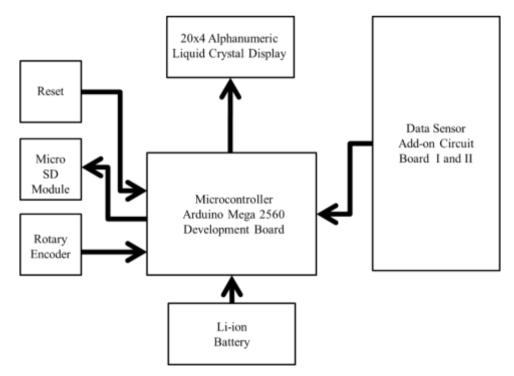
Figure 6 The block diagram of data acquisition system
